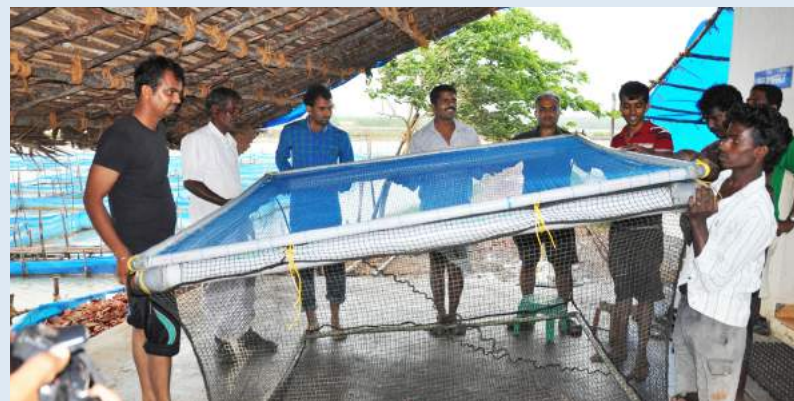
A fully completed grow out cage ready for installation in ponds
