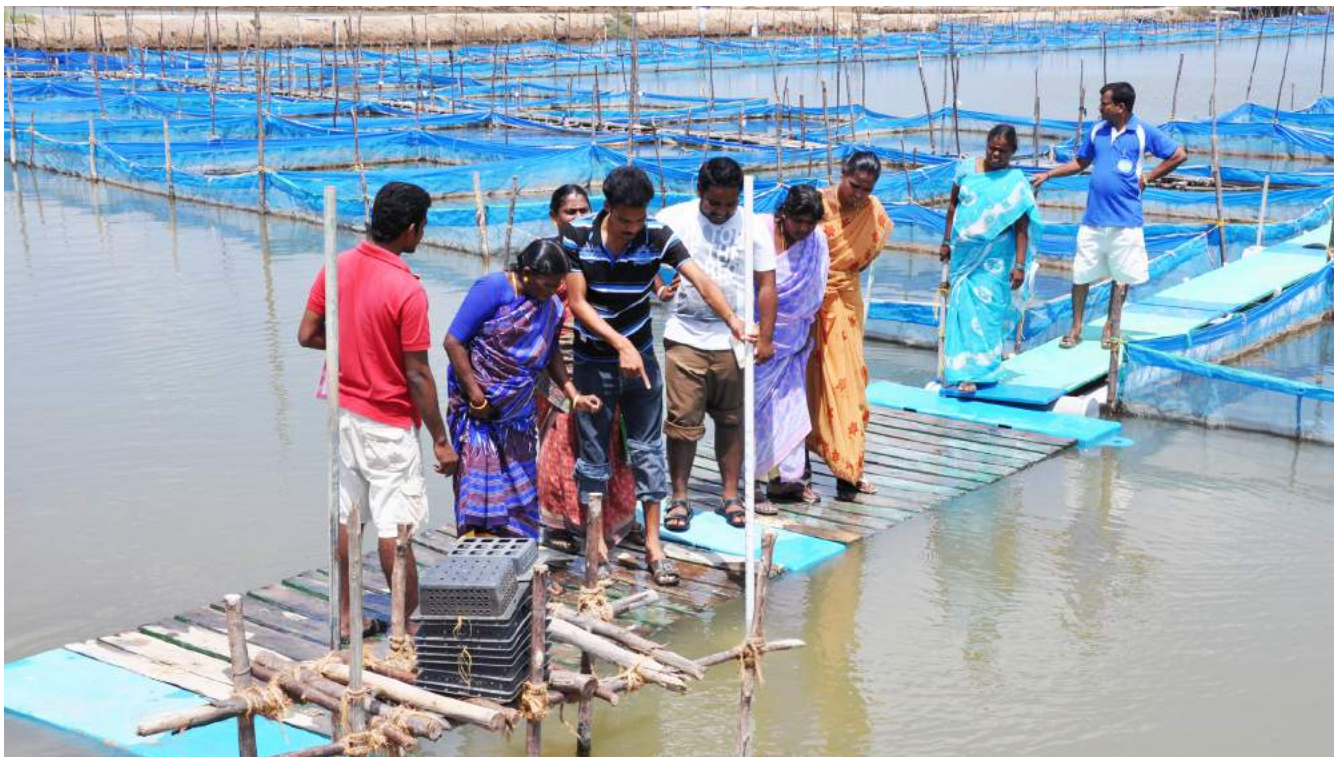
Transparency of water being checked with a Secchi Disc
